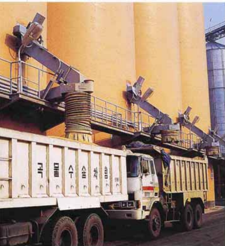
트럭적상차구 / Truck Load-Out Spout
